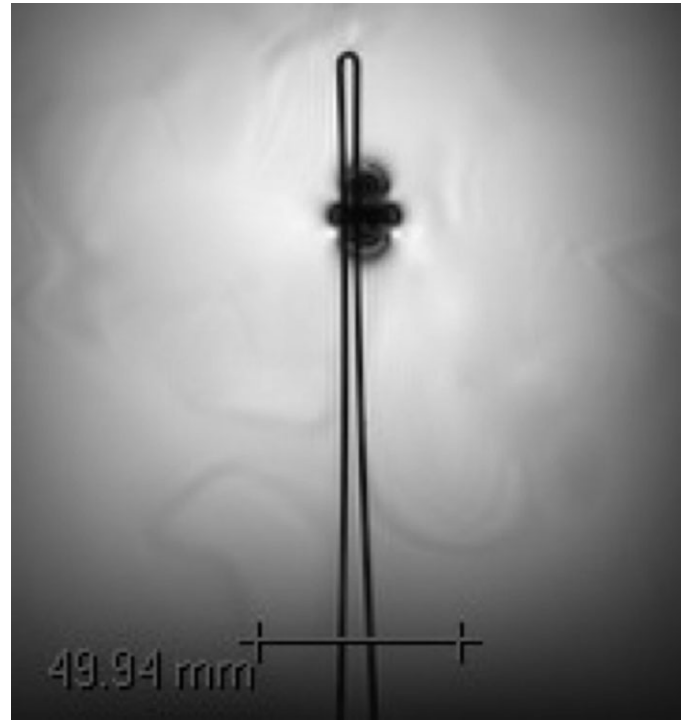
Figure 4. MRI artifacts associated with the wireless lead: short axis view (gradient echo pulse sequence; TR/TE, 100 msec/15 msec; flip angle, 30 degrees; long axis imaging plane).
