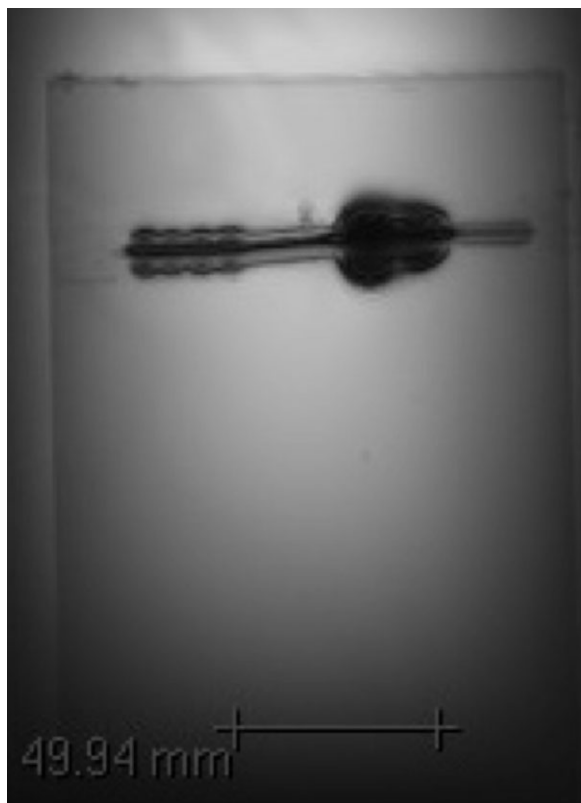
Figure 5. MRI artifacts associated with the wireless lead: long axis view (gradient echo pulse sequence; TR/TE, 100 msec/15 msec; flip angle, 30 degrees; long axis imaging plane).
